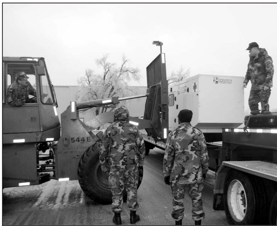
Members of the 190th Civil Engineering Squadron and the 190th Logistics Readiness Squadron load a 100kW generator to support the community health center in Holton, Kan. (Photo by Col. Chris Stratmann)
